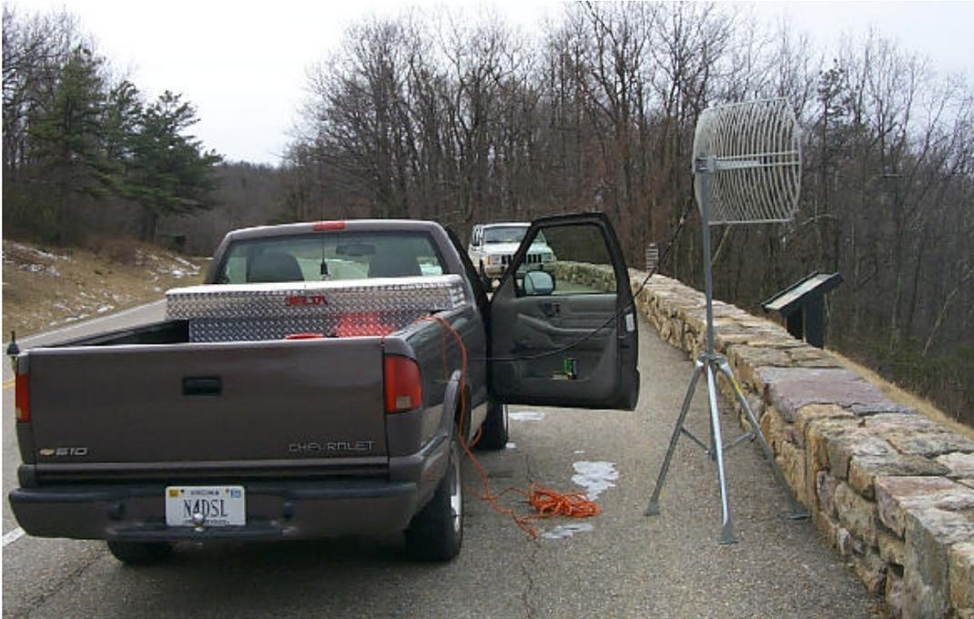
Left: Station N4DSL/p at Two-Mile Run overlook on Skyline Drive. The antenna is pointed northwest at Reddisk Knob, the computer and wireless bridge is on the seat of the truck. Power is provided by a generator in the truck bed.
