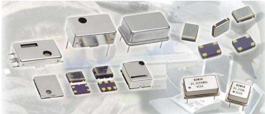
Crystals (XTAL)- Properly cut and mounted a crystal of quartz becomes a Quartz Timing Device, it can be made to bend in an electric field, by applying a voltage to an electrode near or on the crystal. This property is known as piezoelectricity. When the field is removed, quartz will generate an electric field as it returns to its previous shape, this can generate a voltage. Quartz crystal behaves like a circuit composed of an inductor, capacitor and resistor, with a precise resonant frequency.
